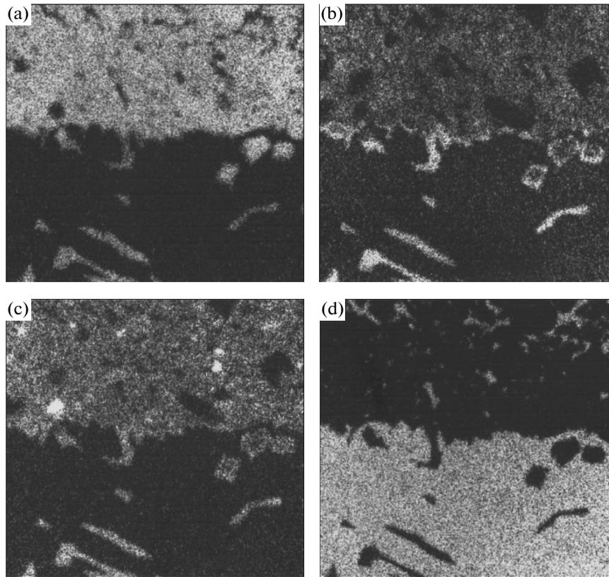
Fig. 5. Images of the contact zone presented in Fig. 4 in characteristic X-ray radiations (a)  $TiK_{\alpha}$ , (b)  $VK_{\alpha}$ , (c)  $CK_{\alpha}$ , and (d)  $NiK_{\alpha}$ .
