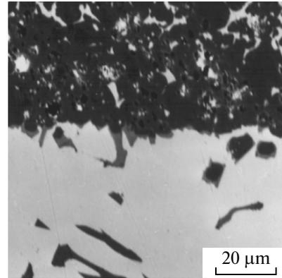
Fig. 4. Electron image of the contact zone of carbonitride  $\text{Ti}_{0.8}\text{V}_{0.2}\text{C}_{0.6}\text{N}_4$  with the nickel melt (1450°C, 1 h).
