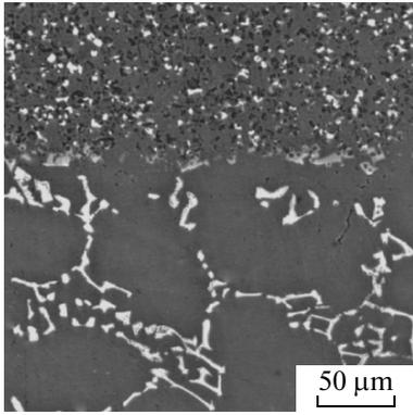
Fig. 3. Microstructure of the contact interaction region in the  $\text{Ti}_{0.80}\text{Hf}_{0.20}\text{C}_{0.6}\text{N}_{0.4}/\text{Ni}$  sample (1450°C, 1 h).
