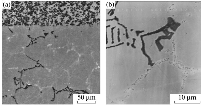
**Fig. 2.** Microstructure of the contact interaction region in the  $Ti_{0.95}Zr_{0.05}C_{0.5}N_{0.5}/Ni$  sample (1450°C, 1 h). (a) General appearance of the contact boundary and (b) fragment of the carbide eutectic.
