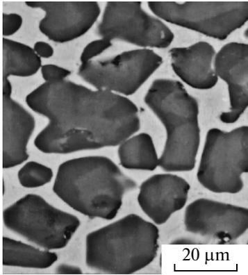
Fig. 6. Microstructure of the grains of the refractory phase in the  $\text{Ti}_{0.95}\text{Mo}_{0.05}\text{C}_{0.5}\text{N}_{0.5}/\text{Ni}$  sample (1450°C, 1 h).
