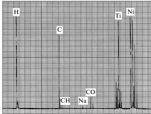
Fig. 1. Mass spectrum of eutectic isolations in the metallic zone of the  $\text{TiC}_{0.5}\text{N}_{0.5}/\text{Ni}$  sample.
