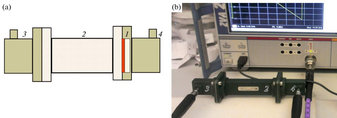
**Fig. 3.** (a) Schematic and (b) photograph of the experimental setup for measuring the reflectance and transmittance of the copper films: (1) substrate with the copper film, (2) waveguide, and (3, 4) coaxial waveguide adapters.
