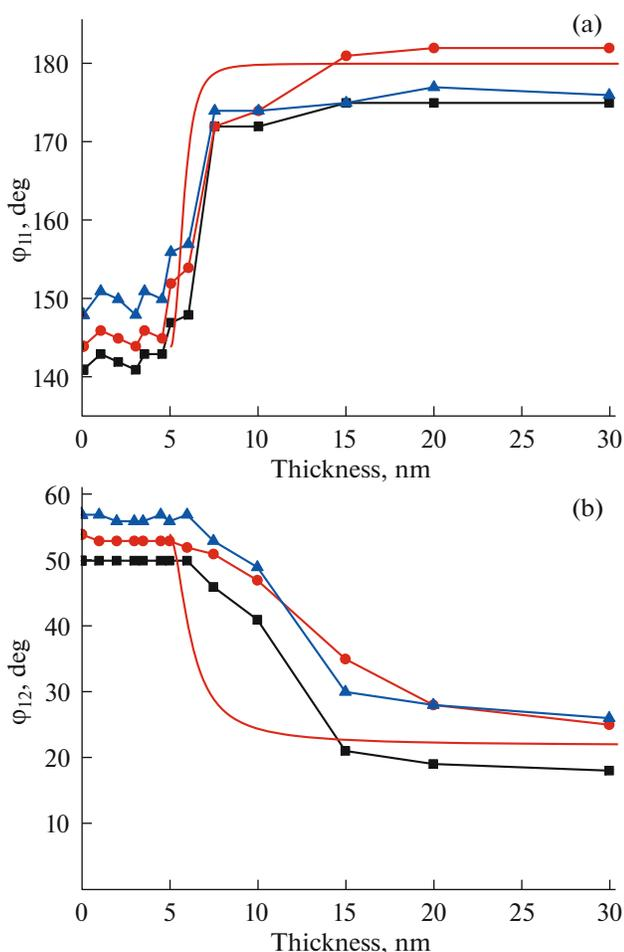
**Fig. 7.** Phase shifts of the (a) reflected and (b) transmitted waves with respect to the incident-wave phase depending on the film thickness. The measurement results at different frequencies are shown by symbols: (■) 9, (●) 10, and (▲) 11 GHz. The calculated data at a frequency of 10 GHz are shown by a solid line. The calculation curves are shifted by a thickness of 5 nm.
