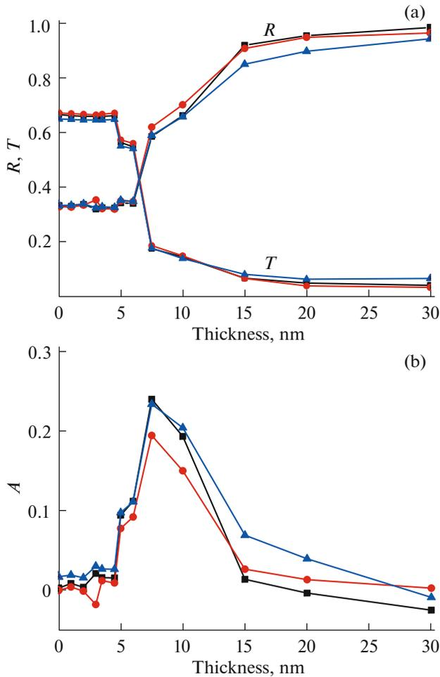
**Fig. 5.** Dependences of the (a) reflectance and transmittance and (b) absorption coefficient on the copper-film thickness measured at frequencies of (■) 9, (●) 10, and (▲) 11 GHz.
