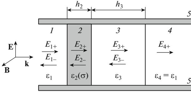
**Fig. 1.** Model used in the calculations: (1, 4) air, (2) copper film with thickness  $h_2$ , (3) quartz substrate with thickness  $h_3$ , and (5) rectangular waveguide.
