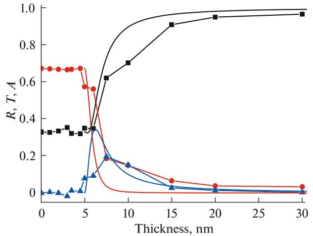
**Fig. 6.** Comparison of the optical coefficients (symbols) measured in the waveguide at a frequency of 10 GHz and (solid line) calculated for the copper conductivity bulk  $\sigma_0 = 5.9 \times 10^7$  Sm/m. The calculated curves are shifted by 5 nm (the copper film thickness at which the continuous conducting layer begins to form).
