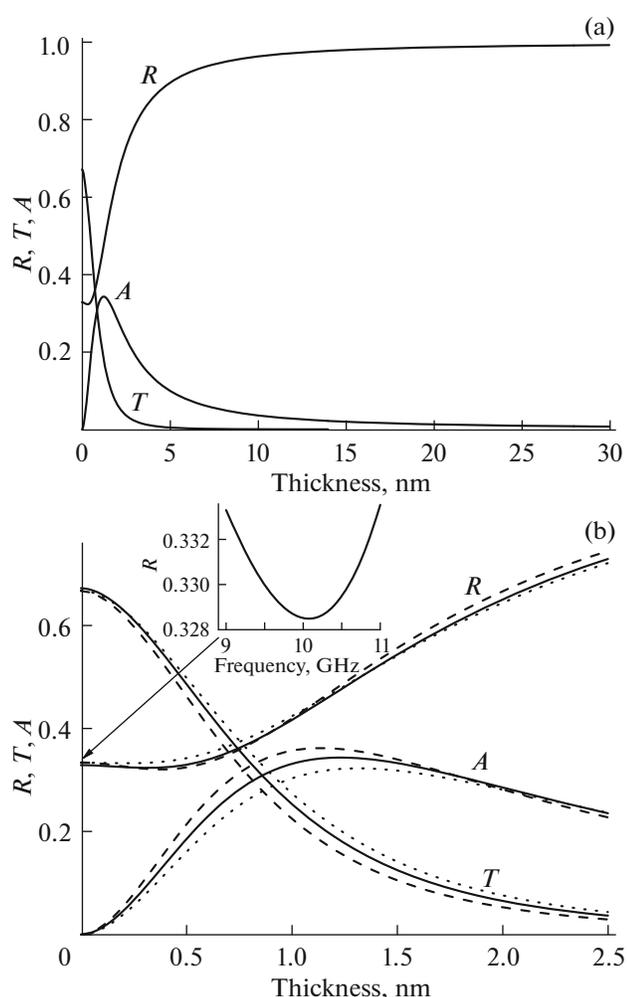
**Fig. 4.** Calculated dependences of the optical coefficients on the copper film thickness (a) at a wave frequency of 10 GHz in the thickness range of 0–30 nm and (b) at frequencies of (dashed line) 9, (solid line) 10, and (dotted line) 11 GHz for film thicknesses from 0 to 2.5 nm. The dependence of the quartz-substrate reflectance on frequency in the range of 9–11 GHz is shown in the inset.
