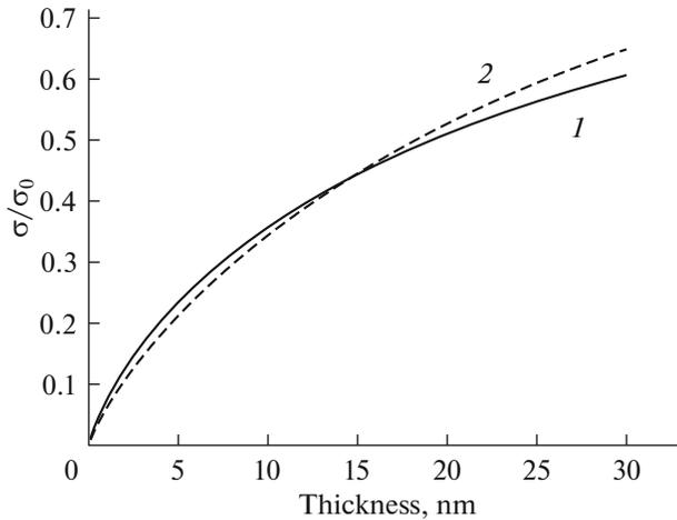
**Fig. 2.** Model dependence of the conductivity of the copper film on its thickness calculated from the exact (curve 1) and approximate (curve 2) formulas.
