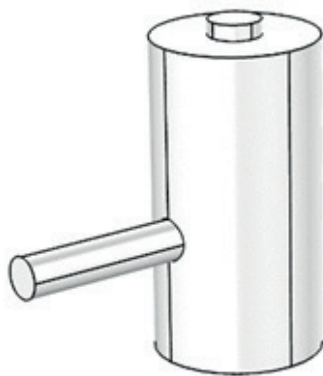
Fig. 1. T-shaped resonator made from Aluminum. The small opening at the top of the resonator is closed by skin of the patient, while the opening at the bottom of the large cylinder is left open. A microphone is mounted at the end on the narrow side cylinder.
