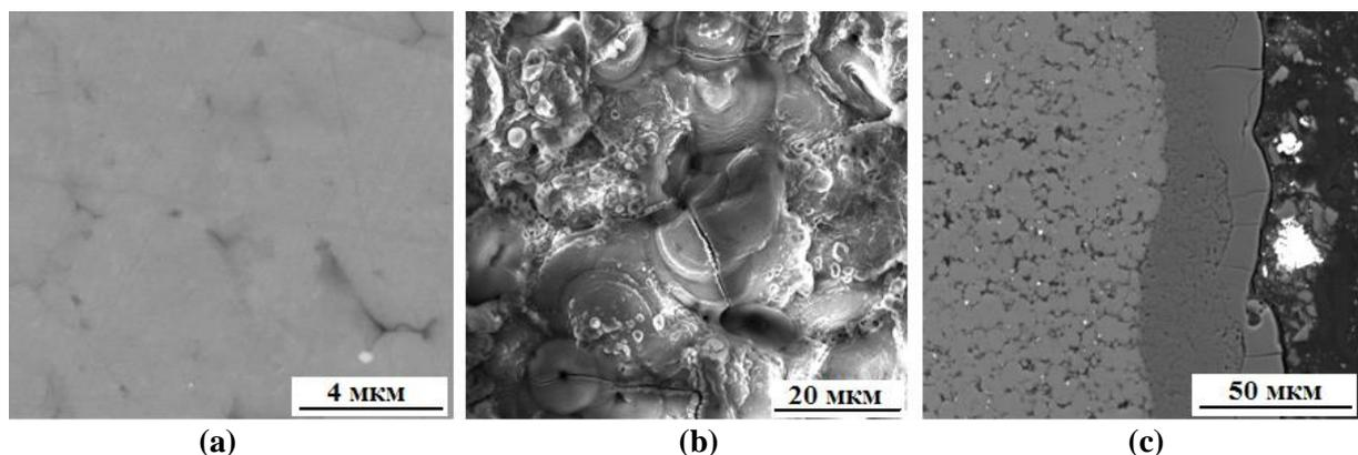
**Figure 1.** SEM images of the aluminum composite without additives (a); the surface (b) and the cross-section structure (c) of the MAO coating obtained for 60 minutes.
