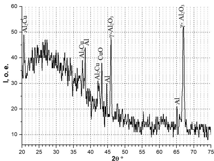
**Figure 4.** X-ray diffraction spectrum of the MAO-coated composite Al-3% Cu after electrochemical tests
