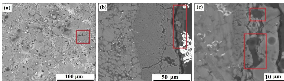
**Figure 3.** SEM images of the surface (a) and cross-section structure (b), (c) of the MAO-coated Al + 3% Cu composite after electrochemical tests in 3% NaCl solution (the areas of the oxide-chloride film are highlighted).
