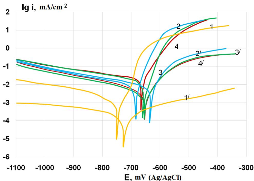
**Figure 2.** Polarization curves of current density  $\lg i$  on potential  $E$  of uncoated composites Al (1), Al + 1% Cu (2), Al + 2% Cu (3), Al + 3% Cu (4) and MAO-coated composites (1'), Al + 1% Cu (2'), Al + 2% Cu (3'), Al + 3% Cu (4') in 3% NaCl at a potential sweep rate of 1 mV/s.
