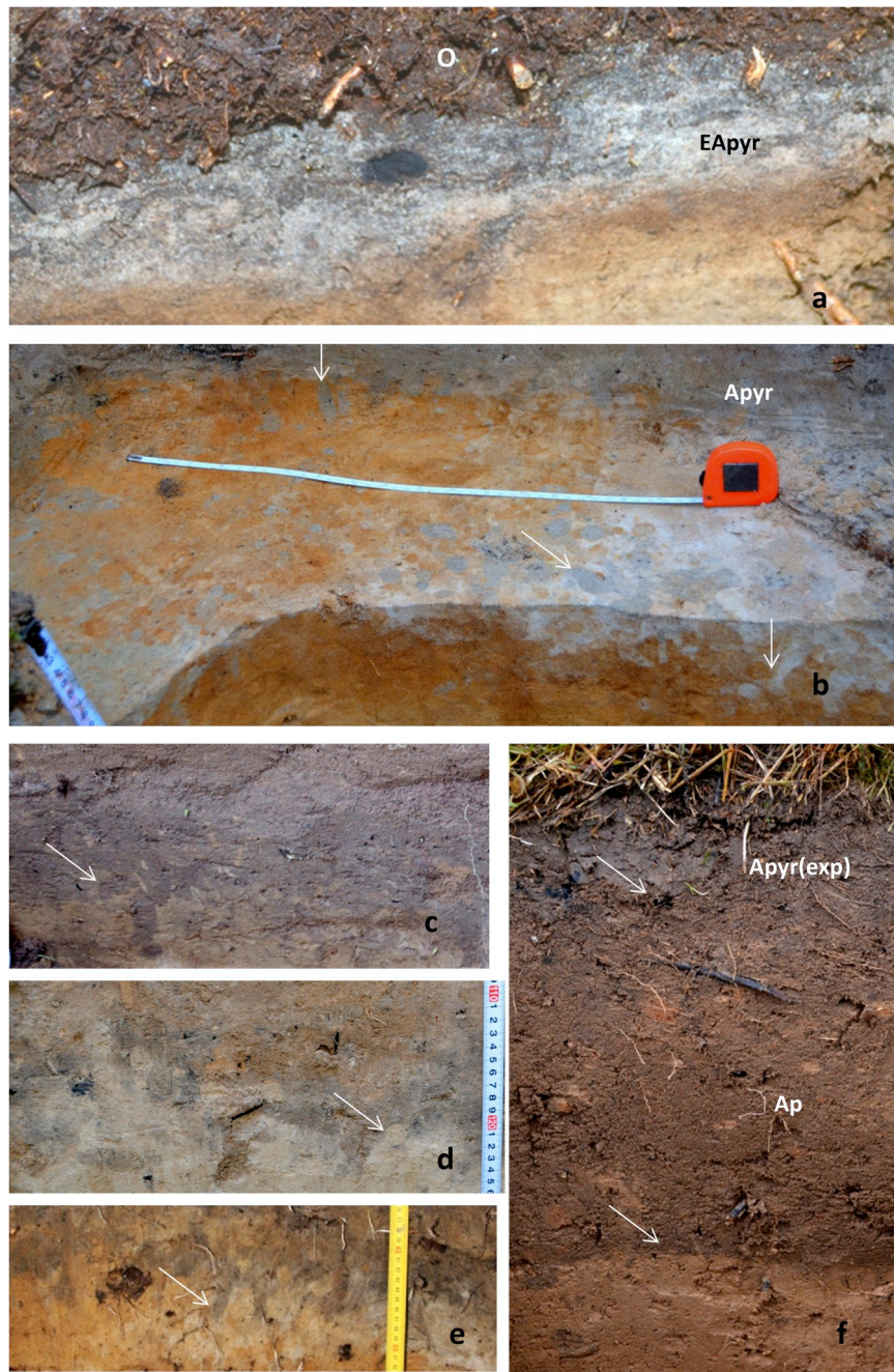
Fig. 5. Lower boundary of organo-mineral layers: (a) lenses of powdered charcoal and bleached mineral soil mass in EApyr, Forest ; (b) traces of fossorial insects on the vertical and horizontal surfaces at the lower boundary of Apyr, Buschland ; (c–e) traces of fossorial insects (digging bees and wasps) in swidden layers: Apyr(1) - Farmland , (d) Apyr(2) - Farmland , Apyr(2) - Buschland ; (f) an even and abrupt boundary of Ap with traces of earthworms and a more gradual boundary of Apyr(exp).
