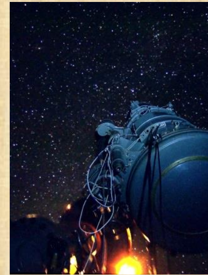
50 cm Maksutov meniscus telescope of the SAI Crimean station used for monitoring of CI Cam
