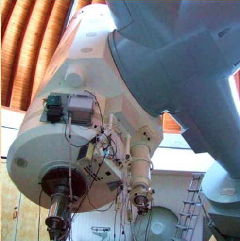
1 m Zeiss telescope of SAO RAS having been mostly used with UAGS spectrograph for medium resolution spectroscopy.
