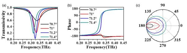
**Fig. 5.** (Color online) Simulation results with different wedge angles of the Teflon prism. (a) The reflectance with different wedge angles 70.7°, 71°, 71.2°, and 71.4°. (b) The phase transitions. (c) The Smith curve.
