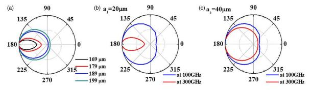
**Fig. 4.** (Color online) Simulation results with different thicknesses of the spacer. (a) Smith curves of the reflectance of the sample for different thicknesses of the spacer. (b) The slit width of  $a = 20 \ \mu\text{m}$  and the layer thickness of  $h = 179 \ \mu\text{m}$ , the Smith curve for the frequency at 0.1 THz and 0.3 THz, respectively. (c) The slit width of  $a = 40 \ \mu\text{m}$  and the layer thickness of  $h = 189 \ \mu\text{m}$ .
