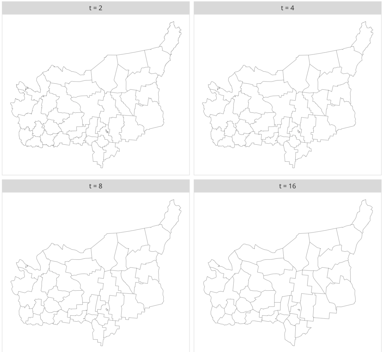
Figure 8: Line generalization with proposed approach. Non-orthogonal parts are generalized with Li-Openshaw (1992) algorithm
