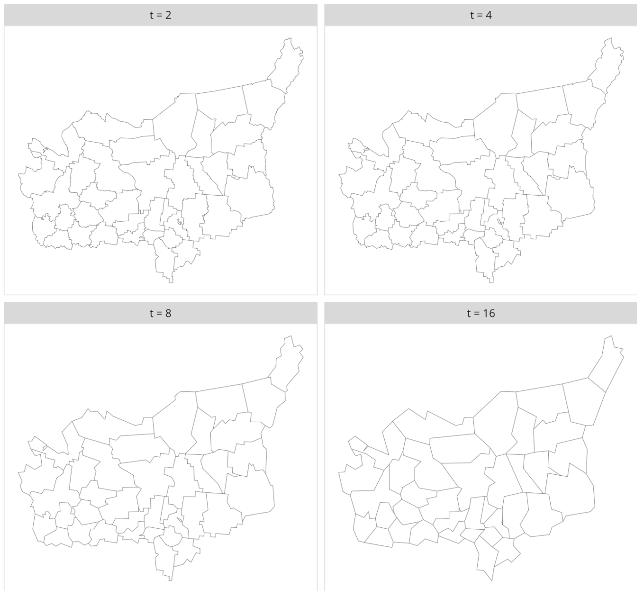
Figure 10: Line generalization with Douglas-Peucker (1973) algorithm
