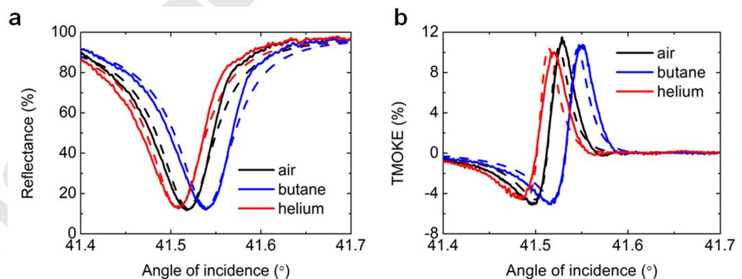
**Figure 3. Reflectance and magneto-optical spectral variations during the gas sensing process.** (a) Reflectance and (b) TMOKE spectra of the sample-1 measured for air, helium and butane as analyte gases. Solid lines correspond to experimentally obtained spectra while dashed lines demonstrate the calculation results. Detailed parameters of the structures are described in Methods.
