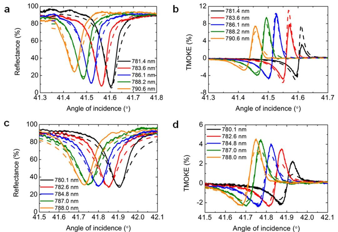
**Figure 2. Ultra-narrow reflectance and magneto-optical resonances in the designed structure.** Reflectance (a,c) and TMOKE (b,d) spectra of the sample-1 (a,b) and the sample-2 (c,d) at different wavelengths. Solid lines correspond to experimentally obtained spectra while dashed lines demonstrate the calculation results. Detailed parameters of the structures are described in Methods.
