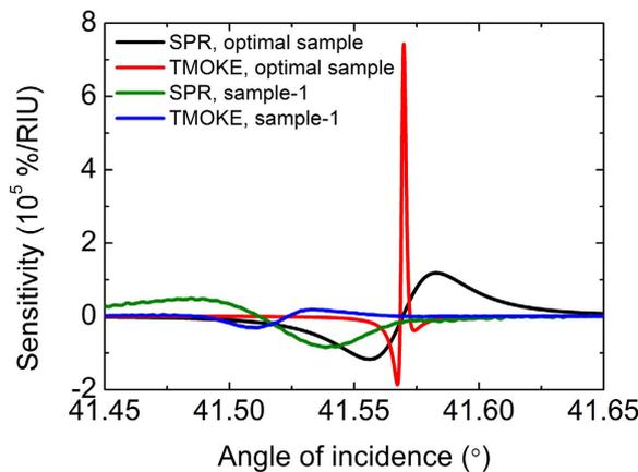
**Figure 4. Comparison of SPR and TMOKE signal sensitivity.** SPR and TMOKE signal sensitivity to the refractive index variation for the sample-1 (experimental data) and a sample with optimized parameters (theory). Detailed parameters of the structures are described in Methods.
