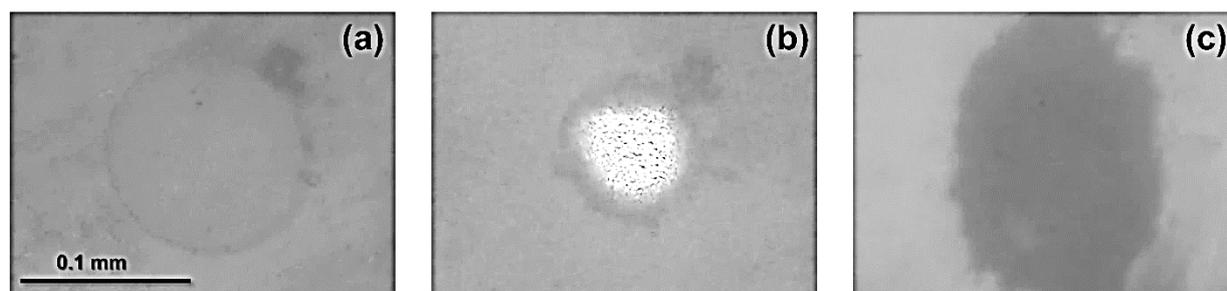
Fig. 1. Microphotographs of the sample (80 wt.% basalt + 20 wt.%  $C_2H_2O_4$ ), taken during experiment in the diamond anvil cell: (a) compressed mixture at 25 °C and 0.8 GPa; (b) decomposition of oxalic acid, 395 °C and 4.0 GPa; (c) coexistence of opaque polymeric phase and silicate phases at 900 °C and 4.7 GPa.
