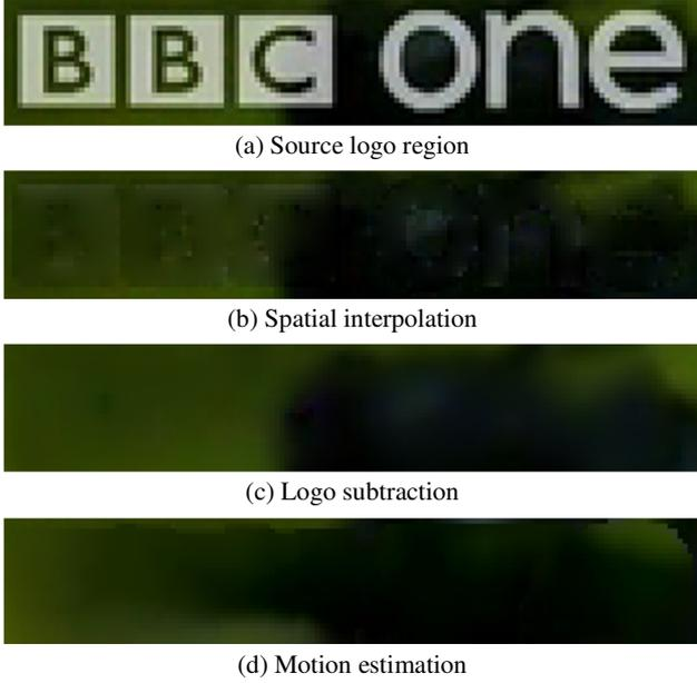
**Figure 4:** Source region and examples of several methods of reconstructing frames
