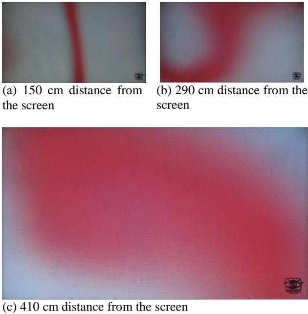
**Fig. 8.** Experimental estimation of the maximum view coverage distance.
