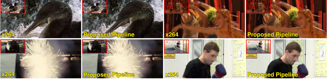
Fig. 5. Compression results of the proposed pipeline and x264 encoder for the same bit rate (1500 kbps). Quality differences between salient and non-salient regions are clearly visible. Degradation of quality for the proposed method in non-salient region has no significant effect.
