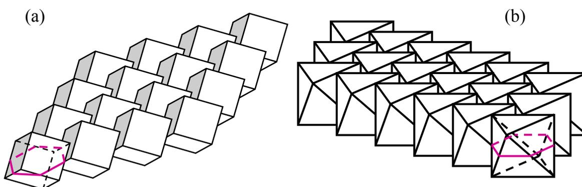
Figure 3. Fragments of assemblies of interlocked cubes and octahedra. (a) Cubes with their space diagonals aligned perpendicularly to the layer. (b) Octahedra resting on their faces. A regular hexagonal middle section is shown for a corner element.
