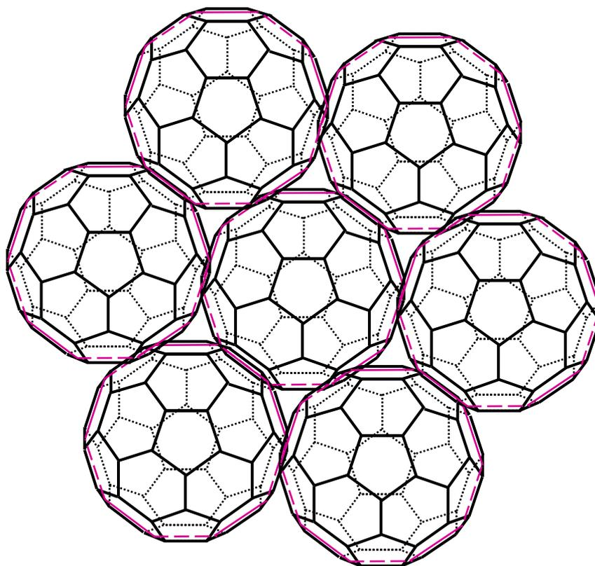
Figure 5. Fragment of an assembly of interlocked buckyballs. The buckyballs are resting on their pentagonal faces. The regular decagons in the middle section are shown in magenta.
