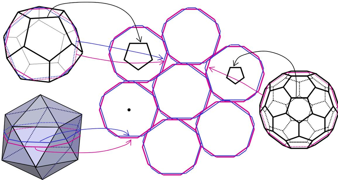
Figure 4. Decagon-based assembly of dodecahedra, icosahedra and truncated icosahedra (buckyballs). Tiling of the middle plane with regular decagons is shown in magenta, a parallel section (upper for the icosahedron and lower for the dodecahedron) is shown in blue. The upper, pentagonal faces of the dodecahedron and the buckyball are shown in black. A black dot in the left part of the decagonal section corresponds to the apex of the icosahedron.
