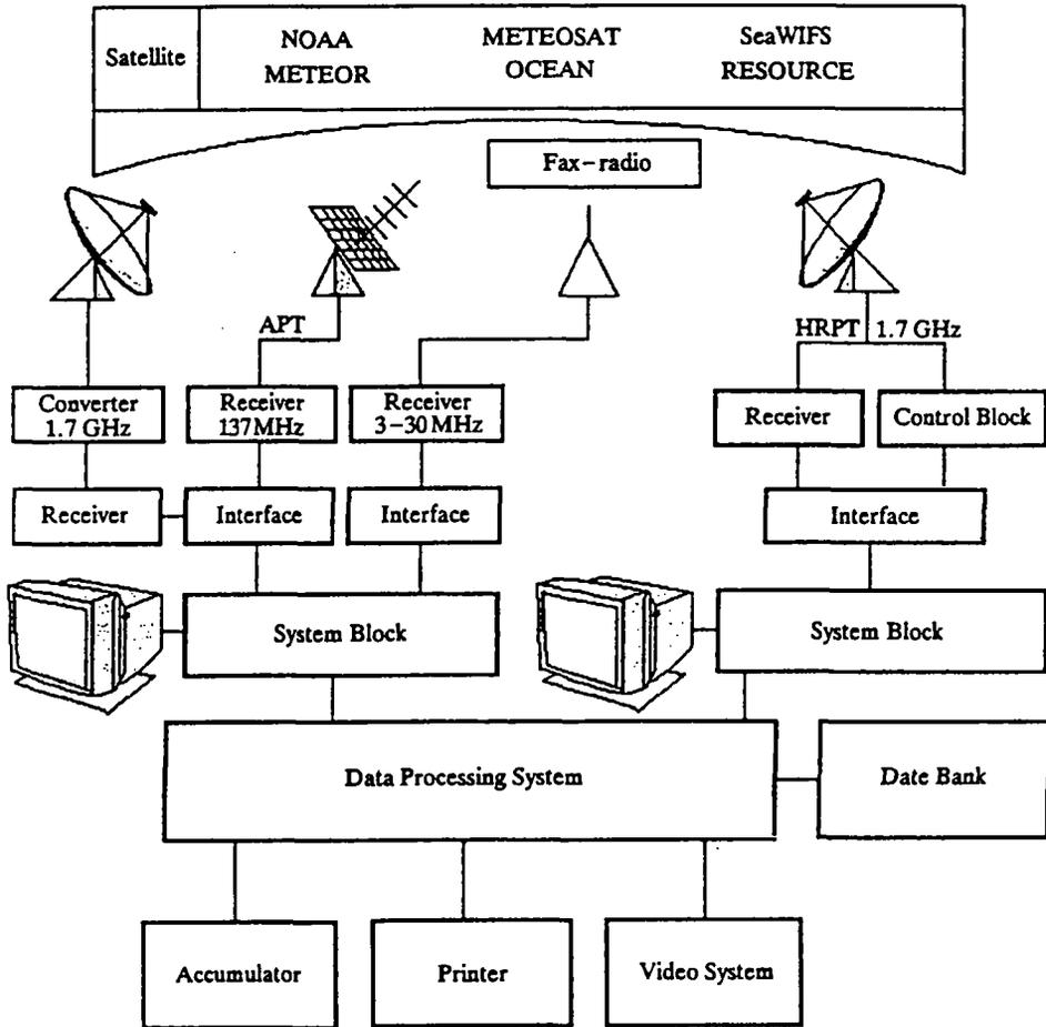
Figure 1. Functional arrangement of the complex for the reception and treatment of satellite and reference data.
