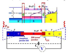
the low potential barrier SIN junctions. For that goal, the TEB with AlOx barrier of height  $U_0$ =1.7 meV should be replaced Cr-based or Ti-based systems with a low potential barrier. Estimation of tunneling probability and imbalance for Pb/Cr<sub>2</sub>O<sub>3</sub>/Pb junction with  $U_0$ =20 meV, superconducting gap  $2\Delta$ =2.7 meV, thickness of the barrier d=5 nm [3] using quantum-mechanical transparency gives Imbalance = 0.7 (!) that is very high figure for TEB [1].
