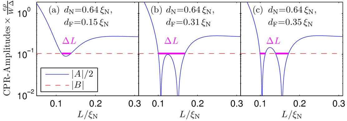
**Figure 2.** The functions  $|A|/2$  and  $|B|$ , based on (28) and (29), as functions of  $L$  for  $d_N = 0.64\xi_N$  and three characteristic values for  $d_F$ . The bold lines marked by  $\Delta L$  correspond to values for  $L$  where the conditions (2) for  $\varphi$  junction realization are fulfilled.
