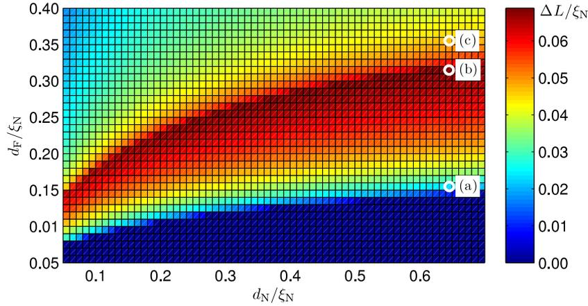
**Figure 3.** The range  $\Delta L$  of possible values for the length  $L$  of the F layer for  $\varphi$  junction realization; it is more sensitive to changes of  $d_F$  than of  $d_N$ . Details for the parameters indicated by white circles are shown in figure 2(a)–(c), respectively.
