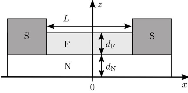
**Figure 1.** The geometry of the considered system. The Josephson junction consists of two superconducting (S) electrodes separated by a ferromagnetic (F) weak link of thickness  $d_F$  and length  $L$ . It is located on top of a thin normal (N) metal film of thickness  $d_N$ .
