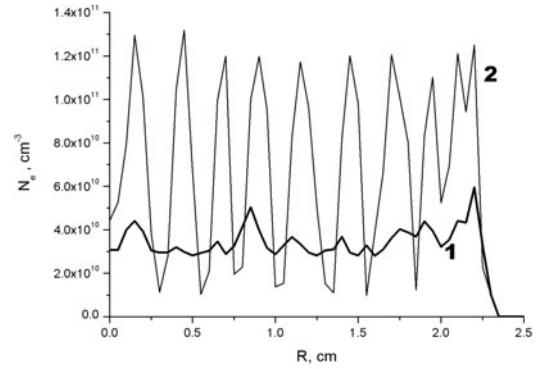
**Fig. 5.** The radial electron concentration distribution averaged over the period (1 –  $\varepsilon = 2$ ,  $l = 0.02$  and 2 –  $\varepsilon = 10$ ,  $l = 0.1$ ).
