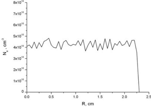
**Fig. 7.** The radial distribution of electron concentration averaged over the period in the atmospheric pressure discharge ( $\varepsilon = 15$ ,  $l = 0.005$  cm).
