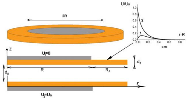
**Fig. 1.** (Color online) The scheme of the simulated DBD discharge.  $Z = 0$  at the upper electrode (grey).
