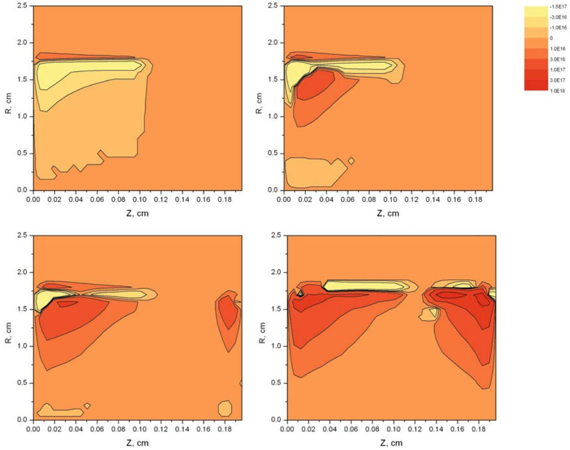
**Fig. 2.** (Color online) The spatial distributions of the radial electron fluxes at different moment of time during the first breakdown (3, 6, 9, 15 ns from the breakdown beginning, respectively).
