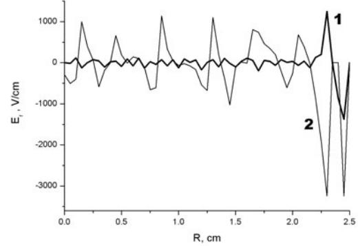
**Fig. 6.** The radial distributions of the radial electric field (1 –  $\varepsilon = 2$ ,  $l = 0.02$  and 2 –  $\varepsilon = 10$ ,  $l = 0.1$ ).
