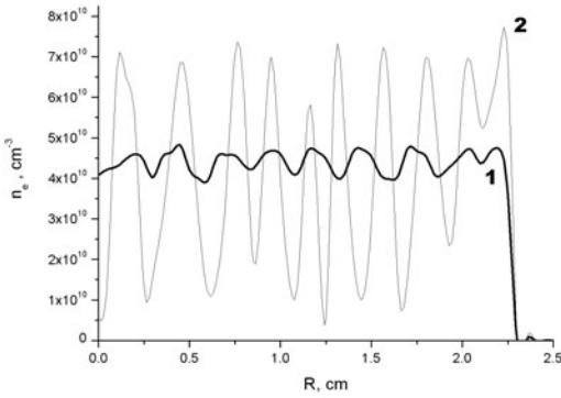
**Fig. 4.** The radial distributions of the electron concentration averaged over the period at different applied voltage frequencies (curve 1–130 kHz and 2–45 kHz).
