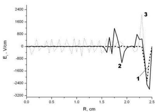
**Fig. 3.** The radial electric fields in the near anode region at first, second and third breakdown, respectively (in the discharge current maximum).
