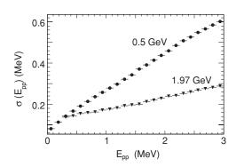
FIG. 5. Resolution of the kinetic energy  $E_{pp}$  of proton pairs, obtained from a simulation.
