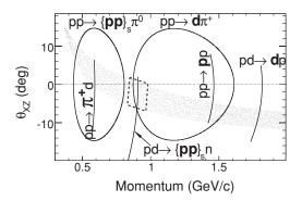
FIG. 2. Single-particle acceptance of the ANKE forward detector at  $T_p = 0.8$  GeV, showing the polar angle projection  $\theta_{xz}$  as a function of particle momentum. The curves show the kinematical loci for different processes (the detected particles are labeled in boldface). For the  $pd \rightarrow \{pp\}_s n$  reaction, the dashed box corresponds to  $E_{pp} <$ 3 MeV and the solid curve is for  $E_{pp} = 0$ .
