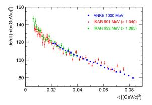
**Fig. 3.** Invariant differential cross section for *pp* elastic scattering. The ANKE data at 1000 MeV with statistical errors (blue squares) are compared to the IKAR hydrogen data at 992 MeV (green circles) [17] scaled by a factor of 1.085 and methane results at 991 MeV (red triangles) [18] scaled by a factor of 1.04. At very small values of |t| there is a rise caused mainly by Coulomb-nuclear interference.
