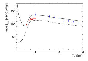
**Fig. 6.** The predictions of Grein and Kroll [16] for the values of the forward pp elastic differential cross section A(GK) (solid line), the corresponding lower limit provided by the spin-independent optical theorem of Eq. (3) being indicated by the broken line. The extrapolated ANKE data, corresponding to the A(Corr.) parameter of Table 2, are shown with their quoted errors by the (blue) circles, whereas the (red) squares are the published IKAR values [17].
