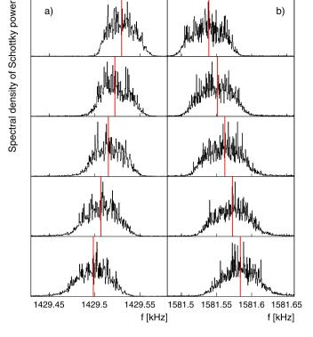
**Fig. 1.** Schottky power spectra obtained during one 300 s cycle and scaled to harmonic number 1 for (a) 1.0 and (b) 2.0 GeV beam energies. Although the data were recorded every 10 seconds, for ease of presentation, only the results from every 60 s are shown, starting from top to bottom. The mean frequencies are indicated by the vertical (red) lines.
