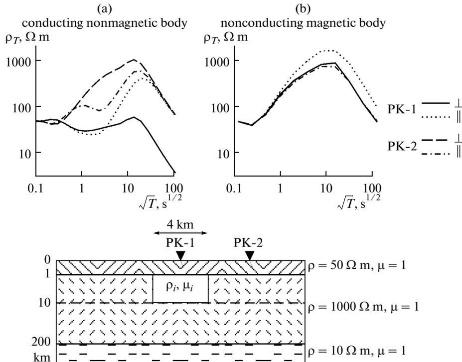
**Fig. 7.** Results of the two-dimensional modeling of the influence of electric conductivity and magnetic permeability anomalies on MTS curves: the geoelectric model (bottom) and the results of calculations for two variants (a)  $\rho_i = 10 \Omega \text{ m}$ ,  $\mu_i = 1$ , and (b)  $\rho_i = 1000 \Omega \text{ m}$ ,  $\mu_i = 3$  (top). The observation points (PK-1 or PK-2) and directions (across or along the anomaly), to which the curves are related are indicated on the right.
