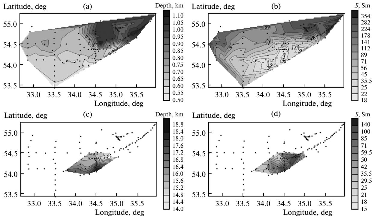
**Fig. 6.** Maps constructed as a result of the interpretation of MT data: (a) depth to the crystalline basement; (b) total longitudinal conductance of the sedimentary cover; (c) depth to the crustal anomaly of electric conductivity; and (d) total longitudinal conductance of the crustal anomaly.
