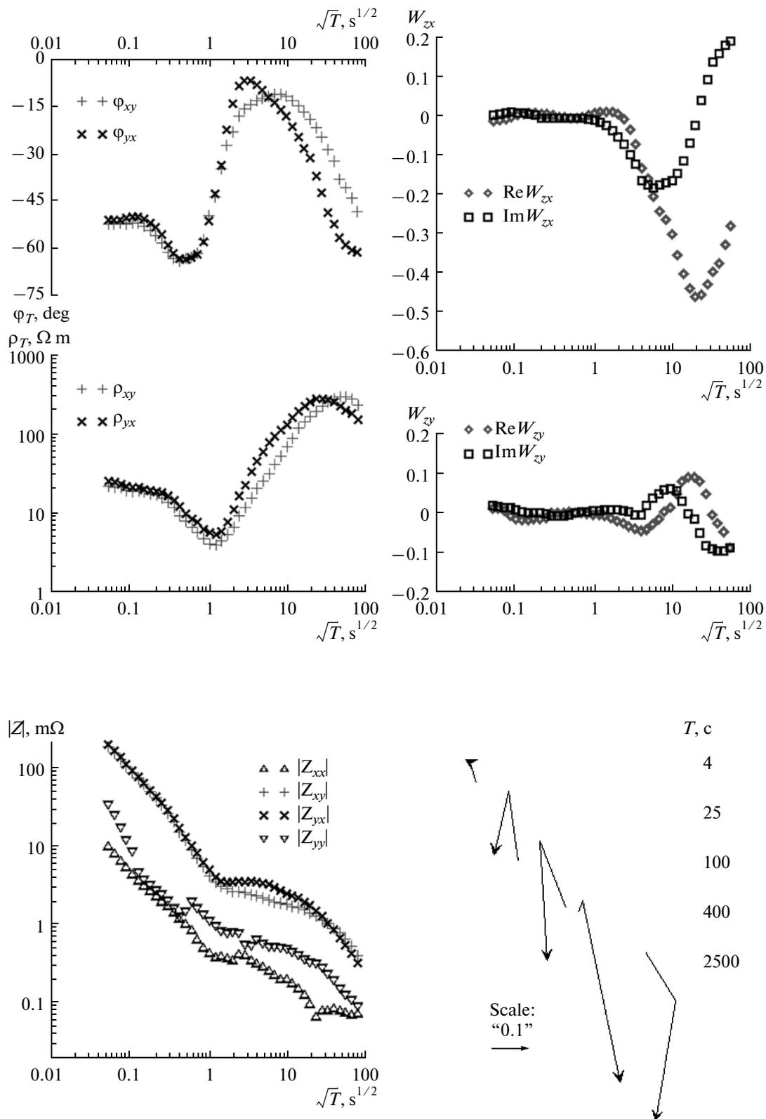
**Fig. 3.** MTS and MVS data obtained at the MSU geophysical base in Aleksandrovska village (ALX stationary point): MTS curves: phases of the main components of the impedance tensor, apparent resistivities, moduli of impedance tensor components (left-hand); and MVS data: real and imaginary parts of tipper matrix components and induction arrows at several periods (right-hand).
