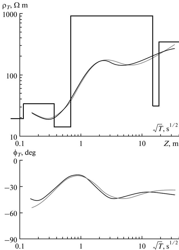
**Fig. 5.** Example of one-dimensional fitting of effective MTS curves of the apparent resistivity (top) and the impedance phase (bottom). Light lines are for observational data, and dark lines are for model data. The upper panel also shows the result of interpretation in the “pseudo-logging curve” form, i.e., as the dependence of the resistivity on depth.
