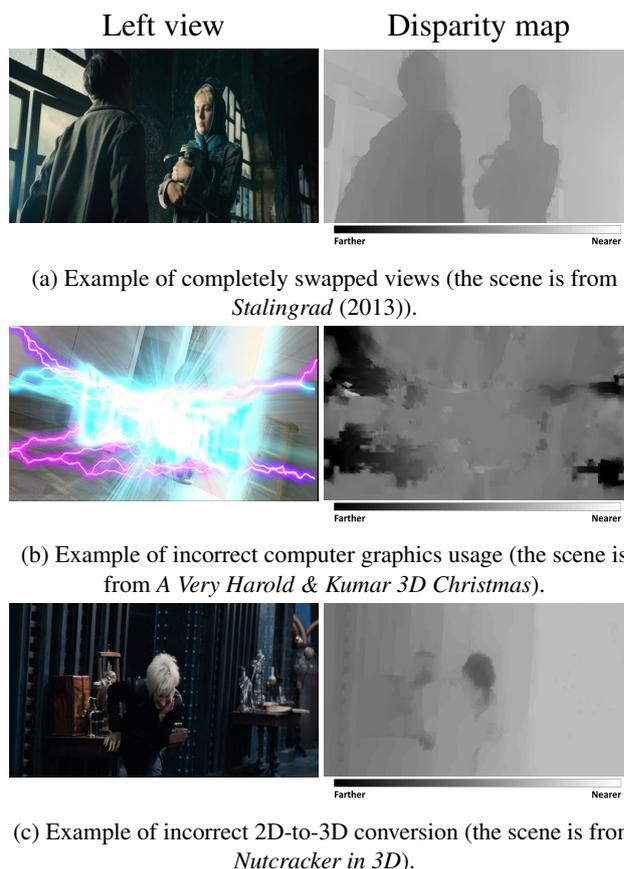
Figure 1: Channel mismatch examples from full-length stereoscopic movies for different stereoscopic video production methods.
