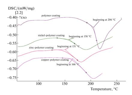
Fig. 1. (Color online) DSC curves of metal-polymer coatings.
