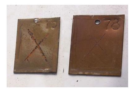
Fig. 4. (Color online) Photos of specimens after salt resistance testing by submerging into a 3% NaCl solution: polymer coating (left) and nickel–polymer coating (right).
