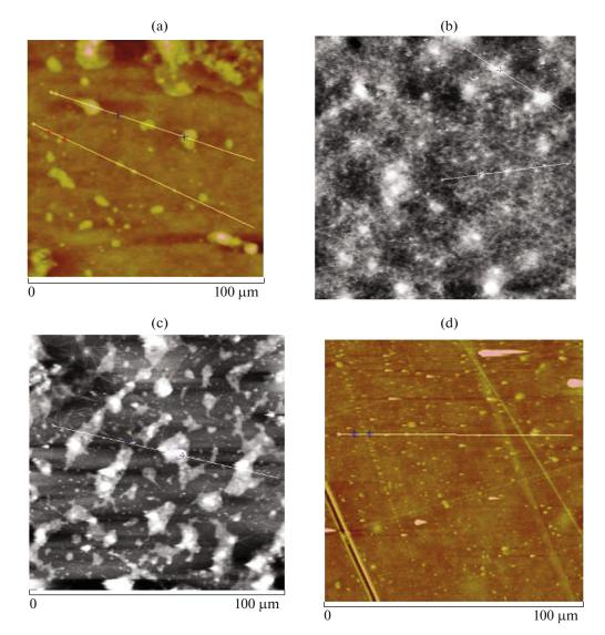
**Fig. 2.** (Color online) Morphology of metal–polymer coatings: (a) nickel–polymer, (b) copper–polymer, (c) zinc–polymer, and (d) polymer.
