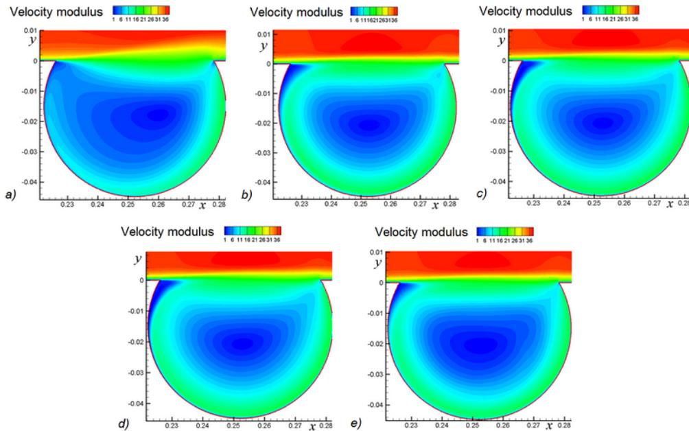
**FIG. 4:** Field of absolute velocity absolute values: (a) SA turbulence model with correction of the source term; (b) realizable  $k-\varepsilon$  model of turbulence; (c) Menter's SST  $k-\omega$  model; (d) transition SST  $k-\omega$  model; (e) Reynolds stress model
