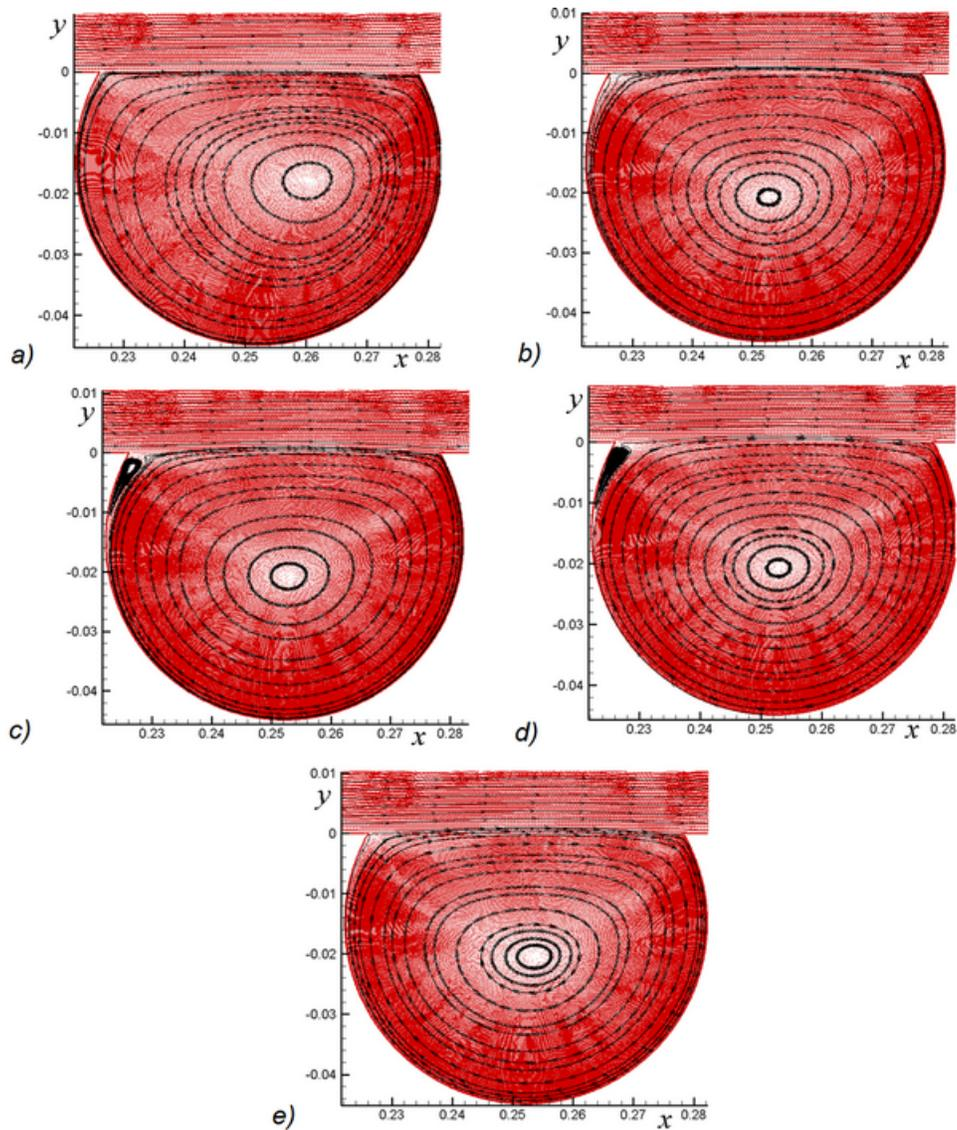
**FIG. 3:** Velocity vectors and paths of the tag particles: (a) SA turbulence model with correction of the source term; (b) realizable  $k$ - $\varepsilon$  model of turbulence; (c) Menter's SST  $k$ - $\omega$  model; (d) transition SST  $k$ - $\omega$  model; (e) Reynolds stress model
