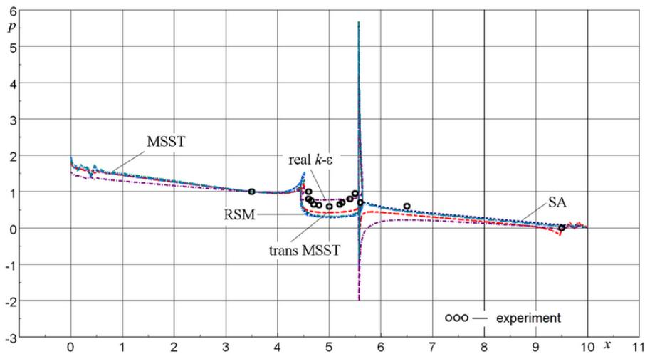
**FIG. 7:** Comparison of the static pressure distribution over the channel wall and the cavity calculated by various turbulence models and the experimental results
