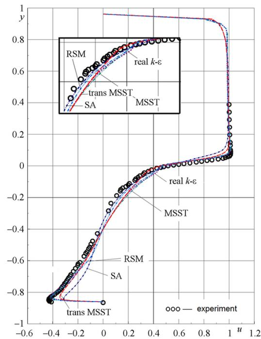
**FIG. 6:** Comparison of the calculation results of the averaged horizontal velocity component and the experimental results obtained by various turbulence models
