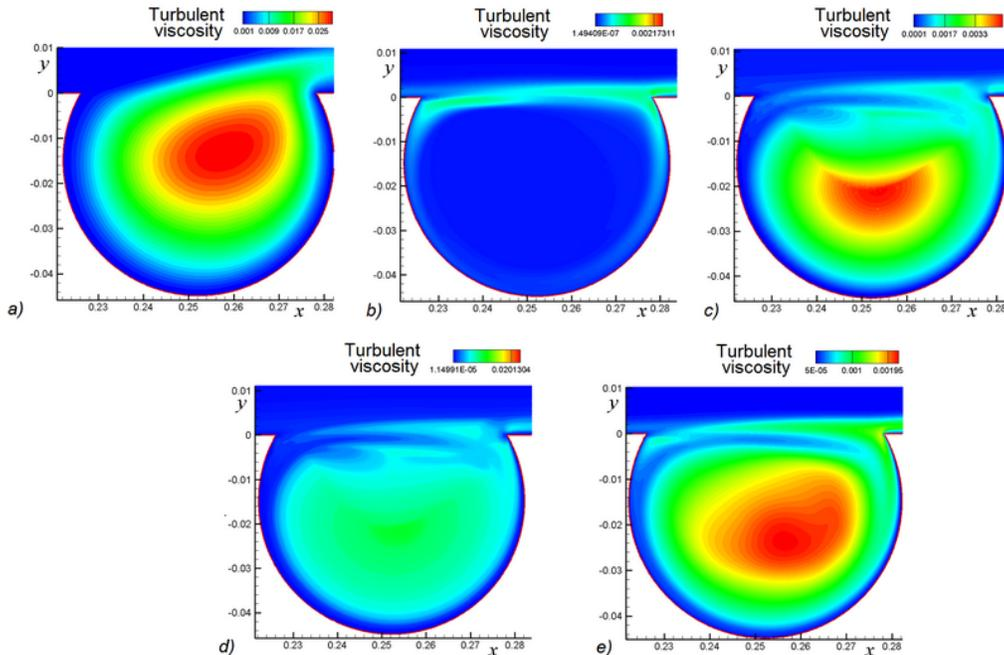
**FIG. 5:** Turbulent viscosity field: (a) SA turbulence model with correction of the source term; (b) realizable  $k-\varepsilon$  model of turbulence; (c) Menter's SST  $k-\omega$  model; (d) transition SST  $k-\omega$  model; (e) Reynolds stress model
