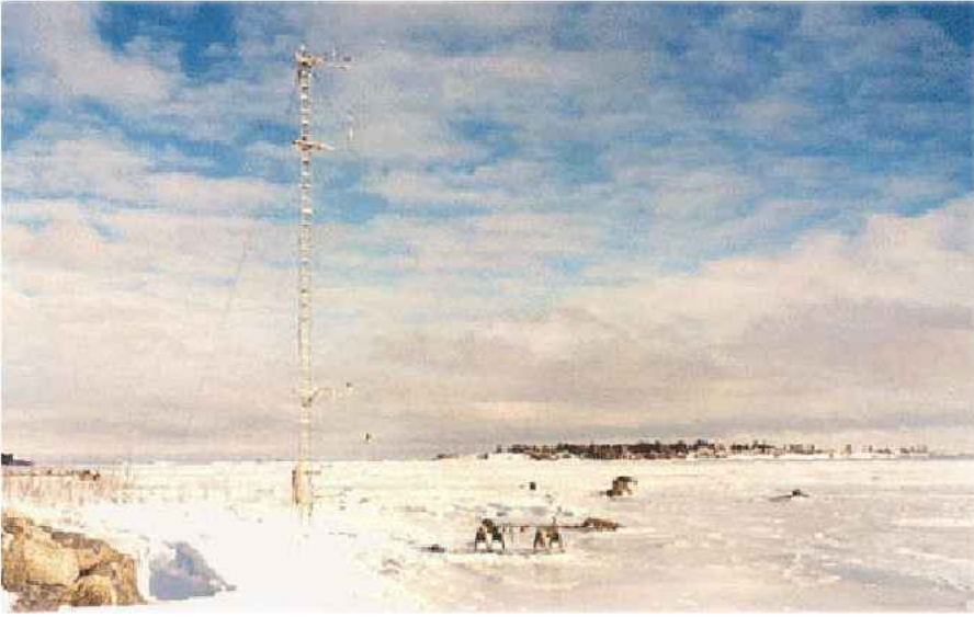
Figure 3. Meteorological 30 m mast on ice at the Umeå station on the Swedish coast of the Gulf of Bothnia.
