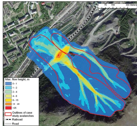
Figure 5: Maximum flow height of case study avalanches calculated in RAMMS using (1) scenario.
