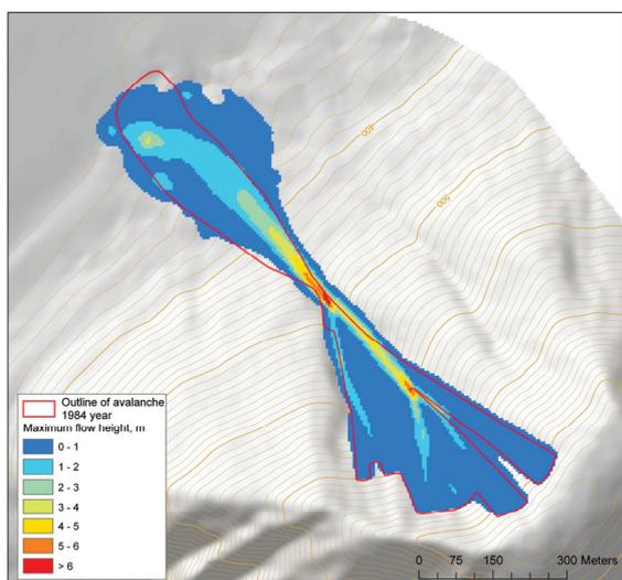
Figure 2: Calculated maximum flow height of an avalanche recorded in 1984 in the № 22 avalanche track.
