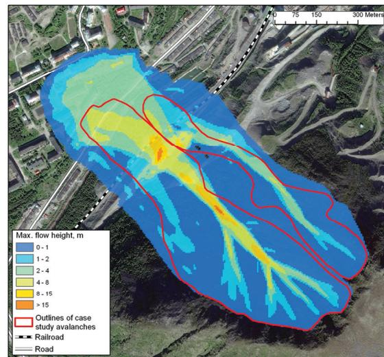
Figure 6: Maximum flow height of case study avalanches calculated in RAMMS using (2) scenario.
