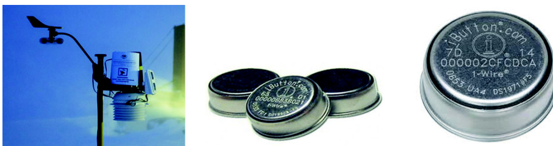
Fig. 1. Automatic meteorological station (AMS) Davis Vantage Pro 2 (on the left), iButton thermal sensors (in the center), and an example of their setup in the course of study (on right).
