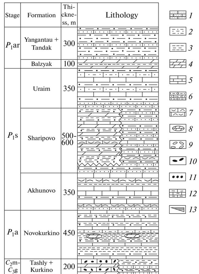
**Fig. 2.** The stratigraphy of the Sim Trough: (1) sandstones; (2) siltstones; (3) mudstones; (4) marl; (5) limestones; (6) calcareous sandstones; (7) detrital limestones; (8) marl concretions; (9) conglomerates; (10) chert concretions; (11) gravel; (12) clayey limestones; (13) olistostrome.
