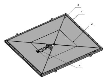
**Fig. 3.** The design of the muon detector: 1 - counter frame, 2 - scintillator, 3 - wavelength shifting bars, 4 - PMT. The size of the active surface is  $1 \times 1 \text{ m}^2$ .
