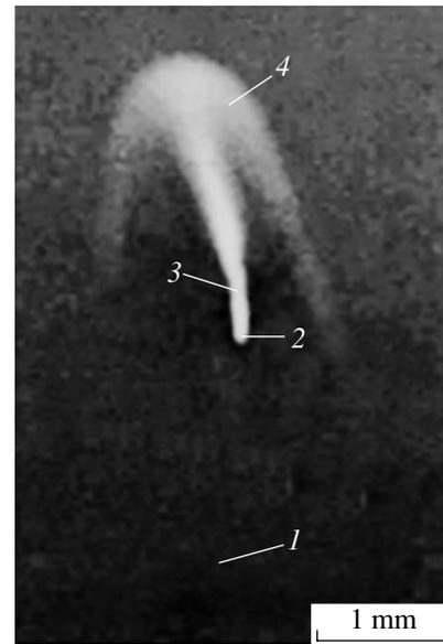
**Fig. 2.** Photographic image of a bleached zone of the OLC/DMF suspension: (1) intact suspension; (2) zone of interaction between focused laser radiation and the suspension (laser beam propagates perpendicularly to the figure plane); (3, 4) bleached fraction of suspension rising up and expanding due to thermal convection.
