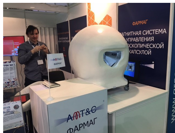
Fig. 8. Acting prototype of electromagnetic system for control of endoscopic capsule designed by Pharmag LLC (AMT&C Group), Russia [10].
