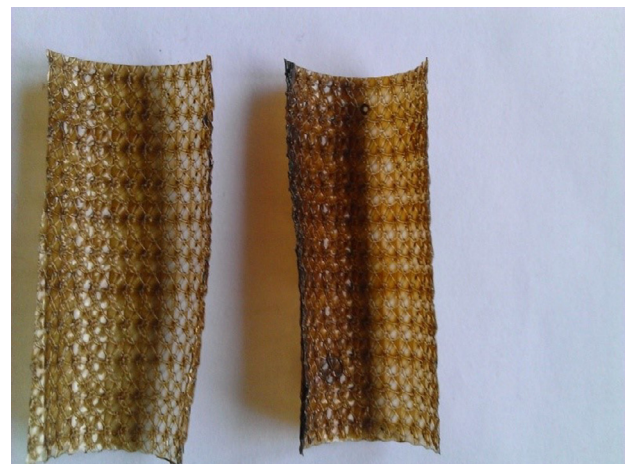
Fig. 3. Samples of mesh implants. The coating of magnetic nanoparticles and tungsten nanoparticles (LbL deposition method) (see text for details).
