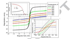
**Figure 2.** Magnetization curves of LSMO nanoparticles at various temperatures. The inset in the upper left corner shows the ZFC-FC curves (the static magnetic field was 100 Oe). The inset at the lower right shows the zoom of the low field region.
