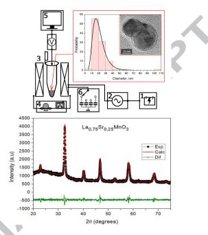
**Figure 1.** a) Equipment for SAR measurement.1. Power supply; 2. generator; 3. solenoid; 4. water cooling system; 5. data acquisition and monitoring system, 6. reconfigurable capacitor system. Inset: TEM image of  $La_{0.75}Sr_{0.25}MnO_3$  nanoparticles with size distribution histogram b) X-ray diffraction pattern for nanoparticles ( $\lambda$ =1.54056Å). Black dots: experimental data; red line: theoretical data; green line: difference.
