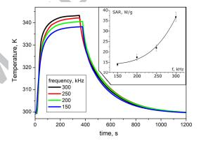
**Figure 3.** The heating/cooling curves of the suspension of LSMO nanoparticles measured at various frequencies. Amplitude of AC magnetic field is 100 Oe. **Inset.** The dependence of SAR on frequency. The dots are experimental data, the curve is a quadratic approximation.
