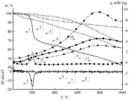
**Fig. 1.** Thermograms, integral curves, and DSC curves for graphite oxide at the heating rate 3 deg/min (1, 5, 9) and for the products of fast thermolysis of graphite oxide (2, 6, 10) and graphite oxide reduced by N<sub>2</sub>H<sub>4</sub>·H<sub>2</sub>O (3, 7, 11) and NaBH<sub>4</sub> (4, 8, 12) at the heating rate 10 deg/min.
