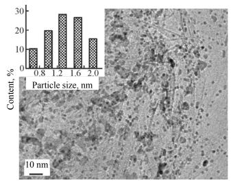
**Fig. 5.** TEM image of the Pt/1 sample. The inset shown the histogram of the Pt particles size distribution.
