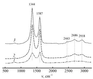
**Fig. 4.** Raman spectra of heat-expanded graphite oxide (1) and heat-expanded graphite oxide reduced by NaBH<sub>4</sub> (2), and N<sub>2</sub>H<sub>4</sub> H<sub>2</sub>O (3).
