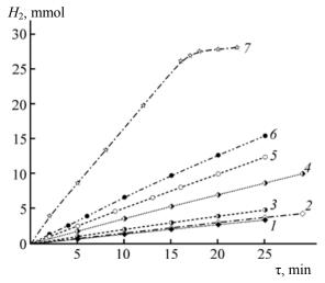
**Fig. 7.** Fragments of hydrogen uptake curves during hydrogenation of nitrobenzene in the presence of Pt compositions based on graphite oxide reduced by  $N_2H_4$ · $H_2O(1)$  and NaBH<sub>4</sub> (2), heat-expanded graphite oxide (4), the Pt/1 (3), Pt/2 (5), Pt/3 (6), and Pt/4 (7) samples. The catalysts contained 0.867 mg (4.44×10<sup>-6</sup> mol) of platinum.
