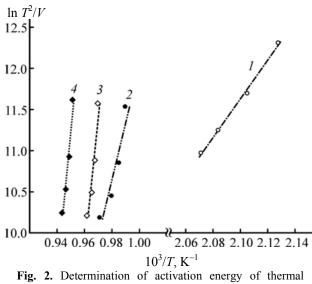
Fig. 2. Determination of activation energy of thermal reduction of graphite oxide (1), heat-expanded graphite oxide (2), and graphite oxide reduced by  $N_2H_4 \cdot H_2O(3)$ , and  $NaBH_4(4)$  using the Kissinger equation.
