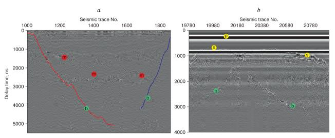
Fig. 3. Examples of radargram obtained on the longitudinal profile at Bezengi Glacier (*a*) and at Chungurchatchiran on Mt. Elbrus (*b*).
