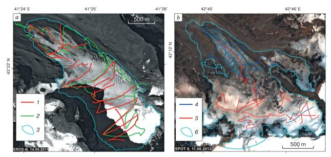
Fig. 1. Ground-based radio-echo sounding and DGPS-survey profiles at Marukh Glacier (*a*) in 2011, and on Djankaut Glacier (*b*) in 2012–2013.
