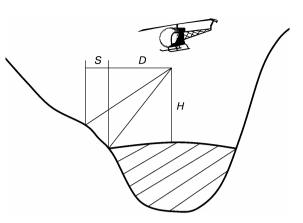
Fig. 5. Schematic representation of identification of coherent reflections (non-target) from mountain slopes during the helicopter-borne RES survey along the longitudinal profile (cf. the text for details).
