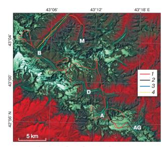
Fig. 2. Airborne radio-echo sounding surveys profiles at the Central Caucasus glaciers in the satellite image Landsat (2011).
