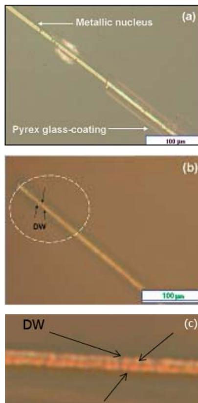
**Figure 1** (online colour at: [www.pss-a.com](http://www.pss-a.com)) Domain pattern pictures for a zone of  $\text{Fe}_3\text{P}$  glass-coated microwires obtained by means of the Bitter technique: (a) microwire dimensions; (b) amorphous state without applied field, (c) with a perpendicular applied field of 350 Oe.
