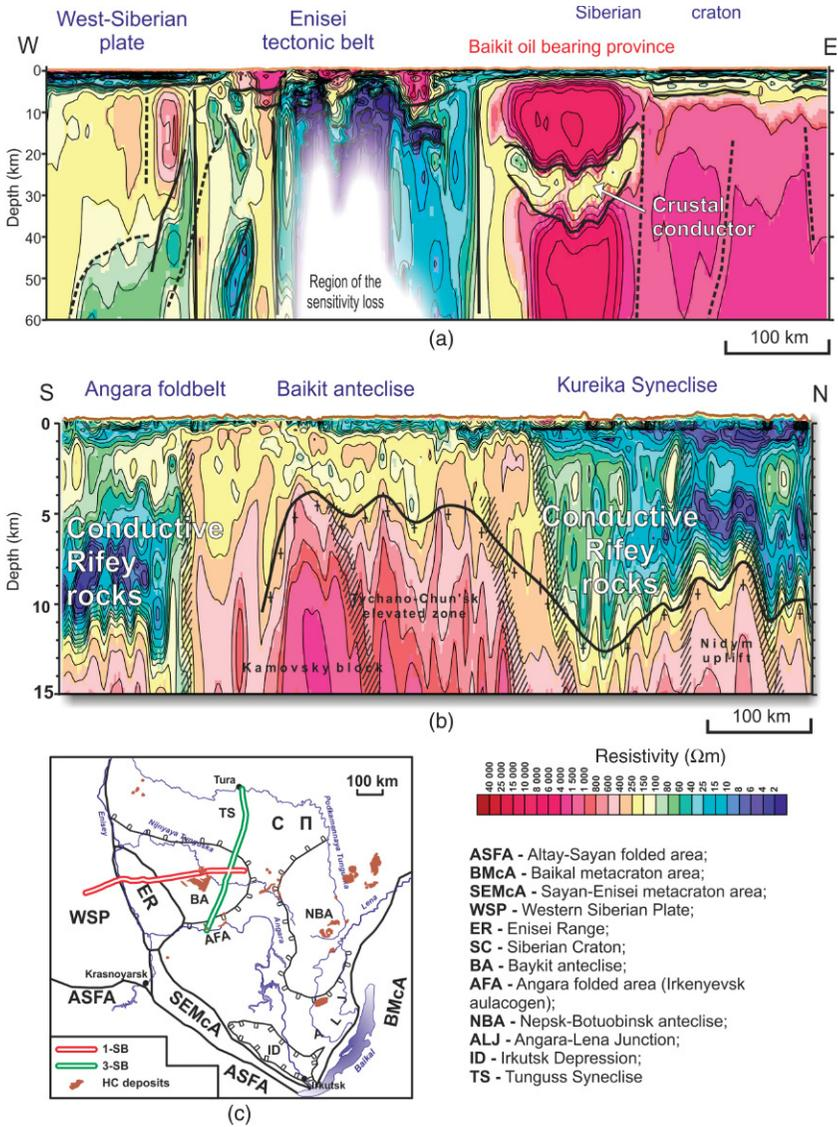
**FIGURE 13.3** Resistivity images along 1-SB (a) and 3-SB (b) geotraverses. Location map is shown in (c).
