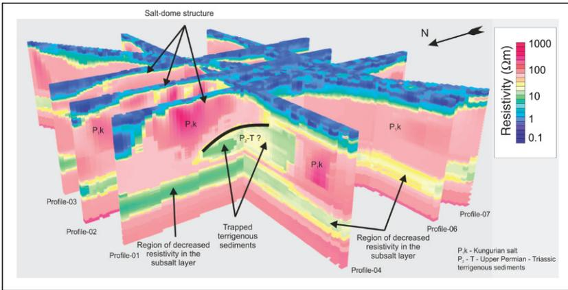
**FIGURE 13.16** 3-D resistivity model of the salt-dome structure.
