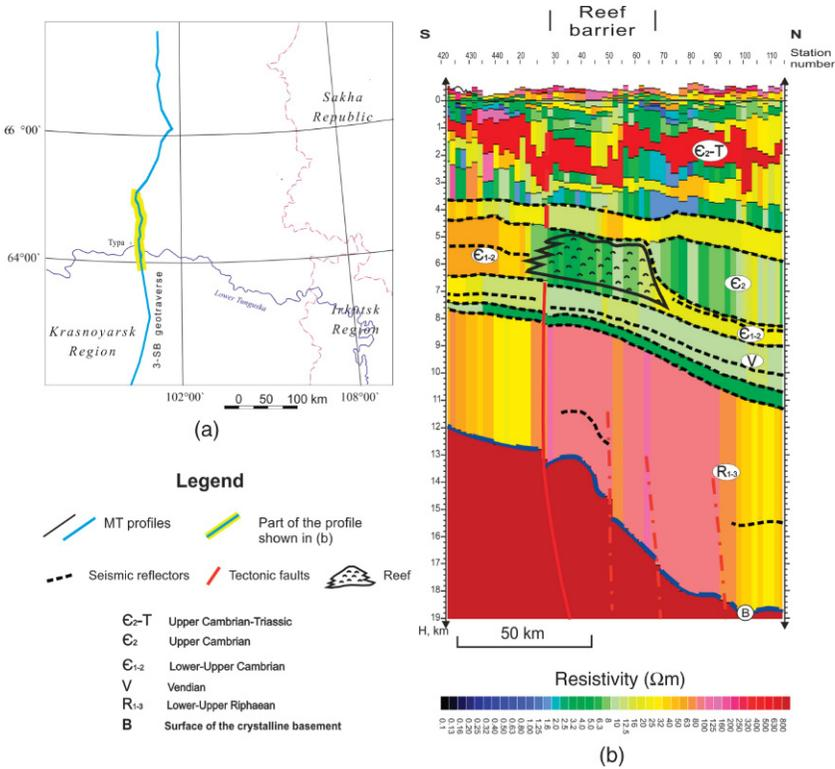
**FIGURE 13.5** Reef barrier in East Siberia as interpreted from MT survey constrained by seismic data.
