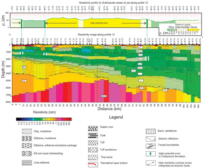
FIGURE 13.7 Resistivity image and reservoir quality distribution along profile 12.
