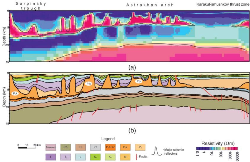
**FIGURE 13.12** Resistivity image along the 1-EV profile obtained from 2-D inversion of MT data (a) compared to seismic-geological model (b).
