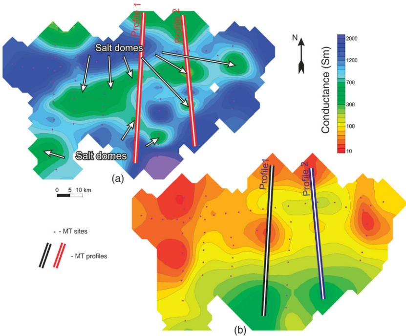
FIGURE 13.14 Signatures of the salt-domes in conductance distributions. (a) 0–4 km depth range; (b) 4–6 km depth range.
