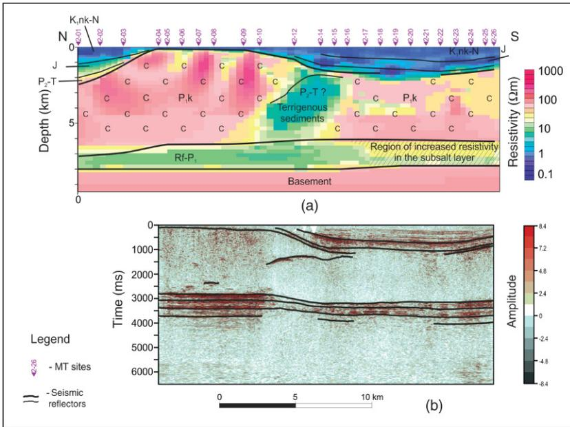
FIGURE 13.15 Salt-dome structure as imaged by magnetotellurics (a) and seismic survey (b).
