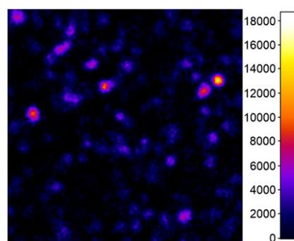
**FIGURE 4** Surface-enhanced coherent anti-Stokes Raman scattering Raman resonant microimage of a sample surface area with a deposition of TNB/Au-NP conjugates (24 μm × 24 μm, fast-mapping, step 0.1 μm). The Raman line at 1,338 cm<sup>-1</sup> of TNB molecules is used [Colour figure can be viewed at [wileyonlinelibrary.com](http://wileyonlinelibrary.com)]
