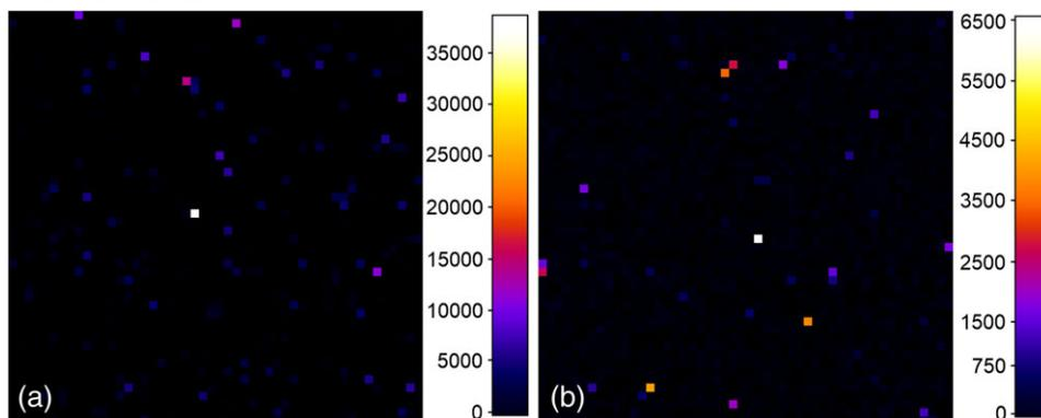
**FIGURE 3** Examples of surface-enhanced coherent anti-Stokes Raman scattering signal spatial distributions for unmodified Au-NPs on CeO<sub>2</sub> film surface (40 μm × 40 μm, slow-mapping, step 0.8 μm): (a) λ<sub>p</sub> = 932 nm; (b) λ<sub>p</sub> = 900 nm. Here and in the following figures, the numbers in the look-up tables correspond to ADC counts [Colour figure can be viewed at [wileyonlinelibrary.com](http://wileyonlinelibrary.com)]
