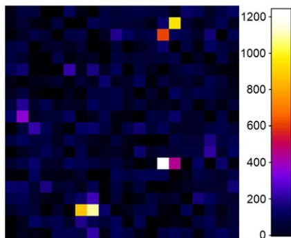
**FIGURE 5** Surface-enhanced coherent anti-Stokes Raman scattering Raman resonant microimage of a sample surface area with a deposition of MPBA/Au-NP conjugates ( $19.3 \mu\text{m} \times 19.3 \mu\text{m}$ , slow-mapping, step  $1.0 \mu\text{m}$ ). The Raman line at  $1,571 \text{ cm}^{-1}$  of MPBA molecules is used [Colour figure can be viewed at [wileyonlinelibrary.com](http://wileyonlinelibrary.com)]
