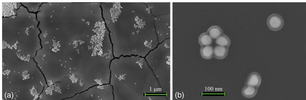
**FIGURE 2** Scanning electron microscope images of a  $\text{CeO}_2/\text{Al}/\text{Al}_2\text{O}_3$  sample surface with the TNB-modified Au-NPs: (a)  $\sim 7.5 \mu\text{m} \times 4.5 \mu\text{m}$  and (b)  $\sim 0.6 \mu\text{m} \times 0.4 \mu\text{m}$  surface areas [Colour figure can be viewed at [wileyonlinelibrary.com](http://wileyonlinelibrary.com)]
