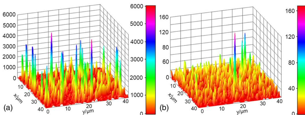
**FIGURE 6** Surface-enhanced coherent anti-Stokes Raman scattering microimages of TNB/Au-NPs on  $\text{CeO}_2$  film surface ( $40 \mu\text{m} \times 40 \mu\text{m}$ , slow-mapping, step  $0.8 \mu\text{m}$ ): (a)  $\lambda_p = 932 \text{ nm}$  (the Raman line at  $1,333 \text{ cm}^{-1}$ ); (b)  $\lambda_p = 900 \text{ nm}$  [Colour figure can be viewed at [wileyonlinelibrary.com](http://wileyonlinelibrary.com)]
