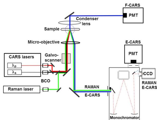
**FIGURE 1** Schematic of the scanning confocal laser micro-CARS spectrometer “Confotec CARS”. Going along the optical axis and overlapping pump, Stokes and epi-CARS beams are shown off-axis for visibility. The micro-objective designated on the picture is in fact the part of the Nikon TE2000S inverted microscope.
