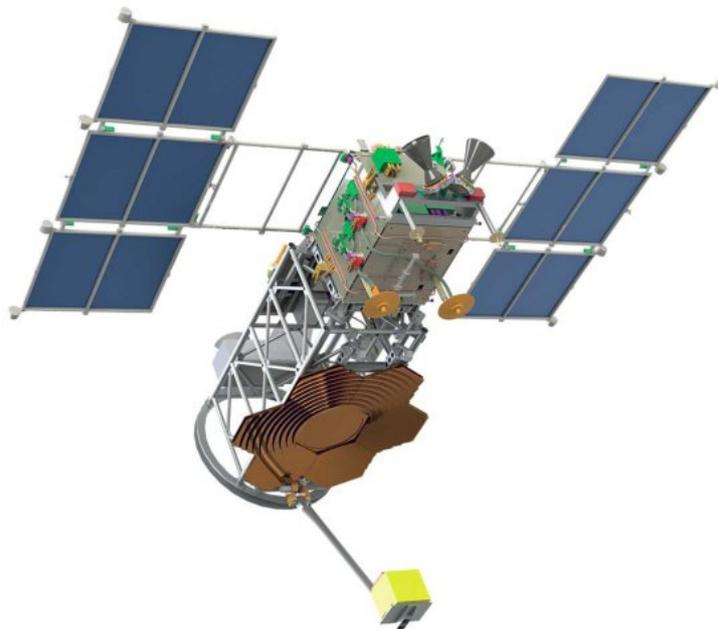
**Figure 1.** Detector TUS on board the Lomonosov satellite.
