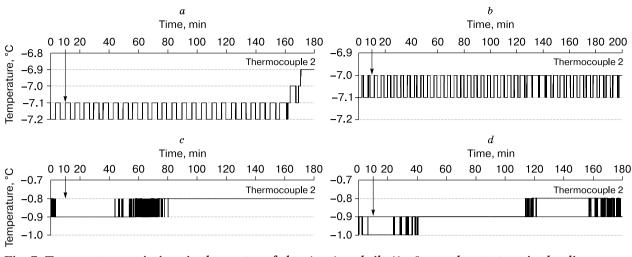
**Fig. 7. Temperature variations in the center of clay** (*a*, *c***) and silt** (*b*, *d***) samples at stepwise loading.** Initial temperatures:  $-7 \degree C(a, b)$  and  $-1 \degree C(c, d)$ . Arrow points to onset of loading.
