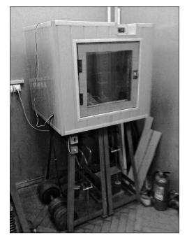
Fig. 1. Cooling chamber and uniaxial compression systems.
