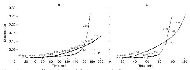
**Fig. 6.** Creep curves of frozen clay (1) and silt (2) at stepwise loading. Initial temperatures:  $-7 \degree C$  (*a*) and  $-1 \degree C$  (*b*). Numerals at the curves are loading steps, MPa.
