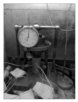
Fig. 2. System for uniaxial compression tests.
