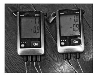
Fig. 3. *Testo-176-T4* temperature loggers and a set of thermocouples.
