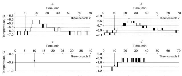
Fig. 5. Temperature variations in the center of clay (*a*, *c*) and silt (*b*, *d*) samples at rapid incremental loading. Initial temperatures:  $-7 \degree C(a, b)$  and  $-1 \degree C(c, d)$ . Arrow points to onset of loading.
