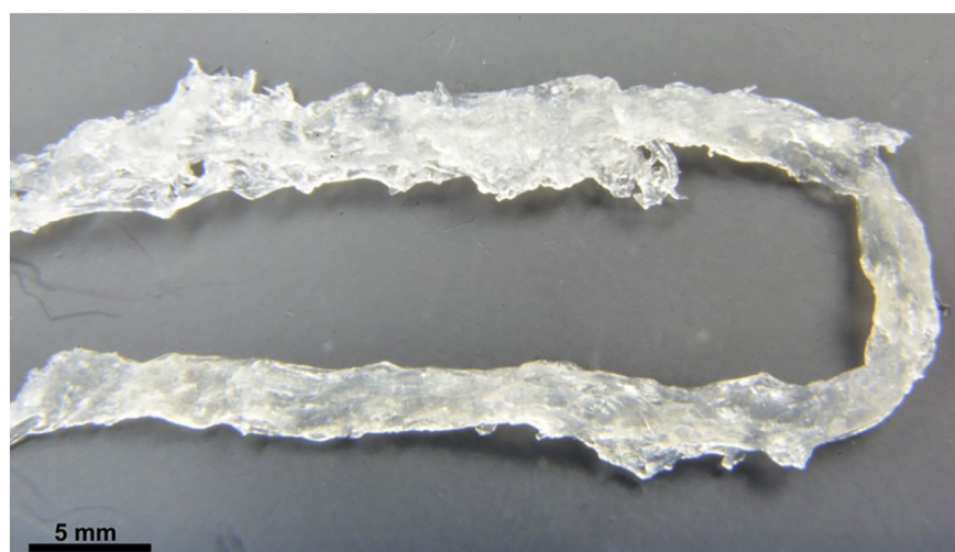
Fig. 2. Completely pigment-free and demineralized scaffold isolated from P. purpurea demosponge still resembles the morphology and the shape of the original collected and freeze-dried sponge (see Supplementary Figure1).
