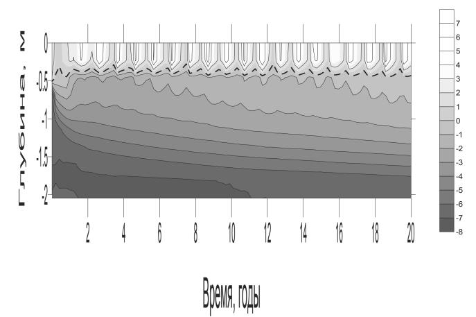
*Fig. 3.* Long-term dynamics of temperature under lake Syrdakh, modeled. Vertical axis is  $-\log_{10}z$ , where z, m; horizontal axis is time, years. Dashed line indicates 0 °C isoterm.
