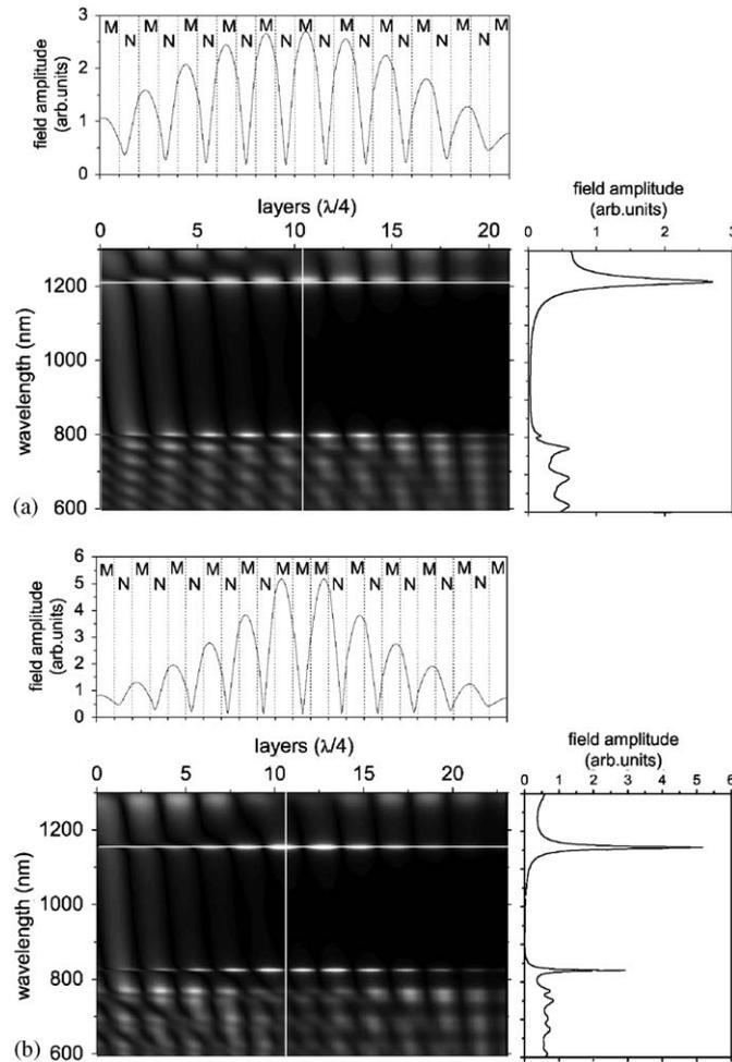
Fig. 2. Spectral dependence of spatial optical field distribution in  $\lambda/4$ -MPC (a) and  $3\lambda/4$ -MMC (b). Field amplitude is shown by grey scale on the patterned plot. White color corresponds to the maxima of the field amplitude. Upper and right plots at each panel represent spatial field distribution at the PBG edge and its spectrum in the central layer taken at cross sections marked by white lines. Magnetic layers are labeled as M and nonmagnetic as N.
