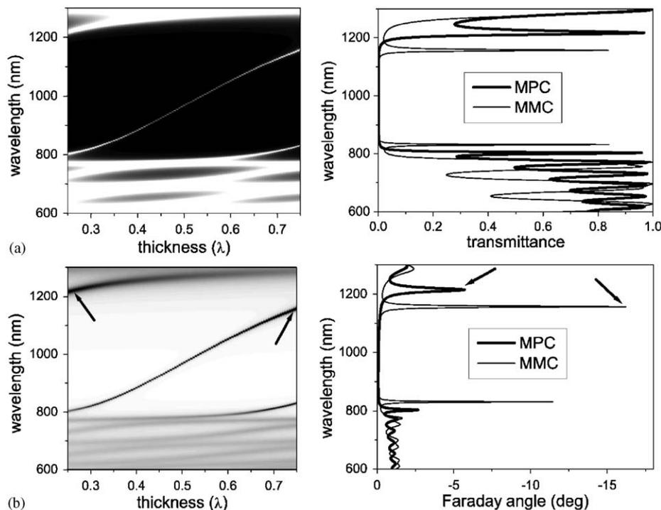
Fig. 1. Set of optical (a) and magneto-optical (b) spectra vs thickness of the cavity spacer. Transmittance and Faraday angle are shown by grey scale on the patterned plot. Right plots show optical (a) and magneto-optical (b) spectra for  $\lambda/4$ -MPC and  $3\lambda/4$ -MMC structures.
