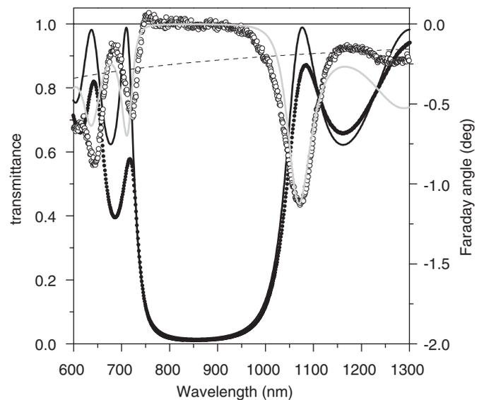
Fig. 3. Optical (filled circles) and magneto-optical (open circles) spectra of MPC measured at the normal incidence and their  $4 \times 4$  matrix technique approximations, black and grey lines, respectively. Dashed line shows magneto-optical spectrum in the case of single Bi:YIG layer with the same thickness of the magnetic material.
